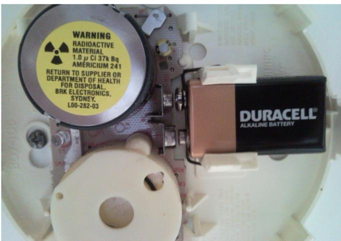
A smoke detector is a device that senses smoke and hence fire. The smoke detectors issue a signal to a fire alarm control panel as part of a fire alarm system, or they issue a local audible or visual alarm. Smoke detectors contain a weak amount of Americium-241 with a half-life of 460 years, which emits alpha particles. The alpha particles ionize the air, so that the air conducts electricity and a small current flows. If there is smoke in the area, it
